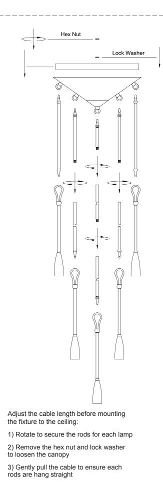
4) Tighten the hex nut and lock washer to secure the canopy
