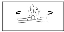
Step.3: Remove 4 wing nuts at bottom side of frame.
