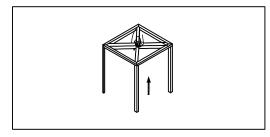
Step.4: Carefully lift metal frame over fixture.
