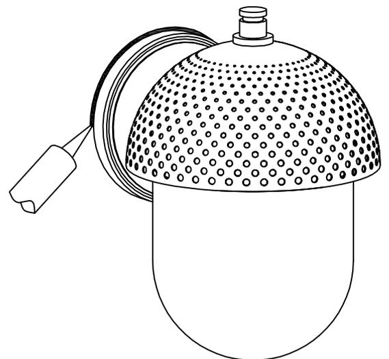
For outdoor use, caulk around fixture with silicone sealant to prevent water intrusion. Leave a gap at the bottom to allow moisture to escape.
