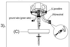
Step.3: Wire fixture to wires in outlet box. Green wire is fo Ground.
