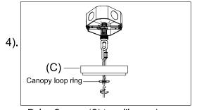
Step.4: Raise Canopy (C) to ceiling and secure with canopy loop ring.
