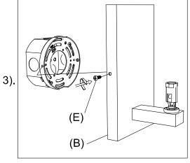
Step.3: Install body (B) to the outlet box and secure with side screw(E). Install Crystal (D) on the body and secure with tube, washer &screw. Place the Candle Tube (C) over the socket and Install light bulb.
