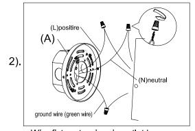
Step.2: Wire fixture to wires in outlet box. Green wire is fo Ground.
