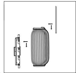
Step.3: Place Cage (D) onto back plate (B) and screw to secure.
