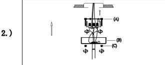
Step.2: Run wire through stems and combine stem lengths to meet desired mounting height. Wire fixture to wires in outlet box. Copper wire is for Ground. Make sure wire is connected to driver before connecting to outlet box. Secure fixture to ceiling using finials (C).
