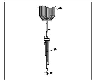
Step.3: Run Stem (D) through Cage (E) and attach Light Cluster (F) to Stem (D). Install G9 LED bulb (G) provided, and carefully lower the cage (E) back over Lamp Cluster (F).
