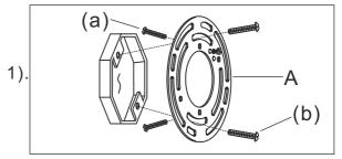
Step.1: Thread the mounting screws (a) into the matching holes in the mounting strap (A). Attach mounting strap (A) to junction box using screws (b).
