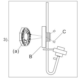
Step.3: Slide body (B) over screws (a) and secure with finials (C). Install light bulb. Place glass (D) over the socket, and then secure glass with screw (E).
