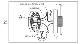
Step.2: Wire fixture to wires in junction box. Copper wire is for Ground.
