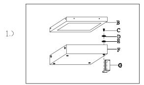
Step. 1. Attach glass (F) to the lamp body (B) by screwing (C) to cap (G) using rubber washers (D&E) provided.
