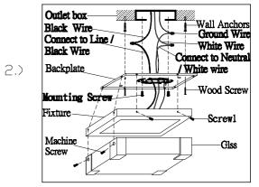
Step.2: Remove mounting bracket (A) from fixture and install to electrical box. Mark where screws at ends of bracket meet the ceiling. Remove mounting bracket from ceiling. Drill holes using 3/16"± drill bit where marked. Install mounting bracket to outlet box and attach anchors to secure bracket at ends. Then wire fixture to wires in outlet box. Copper wire is for Ground.
