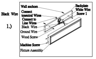
Step.1: Remove mounting bracket (A) from fixture and install to electrical box. Mark where screws at ends of bracket meet the wall. Remove mounting bracket from wall. Drill holes using 3/16"± drill bit where marked. Install mounting bracket to outlet box and attach anchors to secure bracket at ends. Then wire fixture to wires in outlet box. Copper wire is for Ground.
