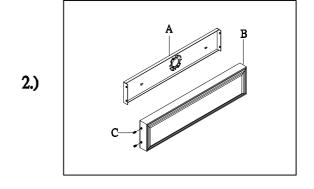
Step.2: Install lamp body (B) to back plate using two screws (C) on the sides.
