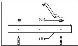
step3:Secure the rod assembly to the set nipple of the canopy as shown in diagram.
