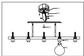
step4:Install fixture to bracket and tighten ball nuts at the ends of the canopy to secure.
