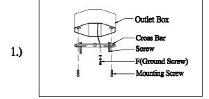
Step.1: Remove mounting bracket from fixture and install to electrical box.
