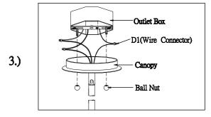
Step.3: Wire fixture to wires in outlet box. Copper wire is for Ground. Install canopy (A) to bracket and tighten ball nuts on the canopy to secure.
