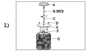
Step.2: Run wire through stems (B&C) as you attach the body (G). Combine stem lengths to meet desired mounting height. Install 3 - G9 bulbs (F),
