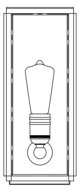
CAUTION: To prevent water intrusion, caulk around back-plate where fixture meets the wall using outdoor silicone sealant. Leave a small gap at the bottom to allow moisture to exit.
