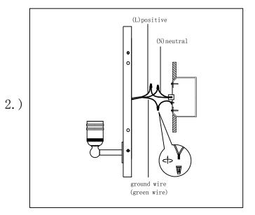
Step. 2: Wire fixture to wires in outlet box. Copper/green wire is for Ground.
