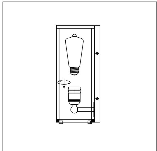
**Step. 4:** Install medium base Edison-style bulb (not included) into socket.
