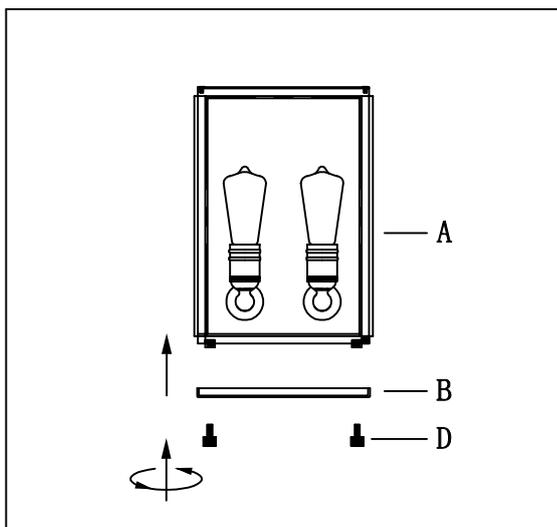
**Step. 5:** Attach bottom cover (B) to the body (A) and tighten screws (D) on the bottom of the fixture to secure.
