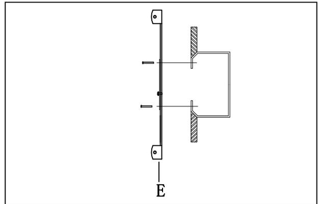
**Step.1:** Install mounting bracket (E) to outlet box.
