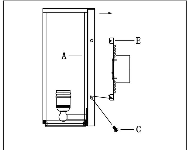
**Step. 3:** Run a bead of silicone sealant along the edge of the backplate to prevent water intrusion. Leave a gap at the bottom to allow moisture to escape. Attach the fixture to the mounting bracket (E) using screws (C) provided.
