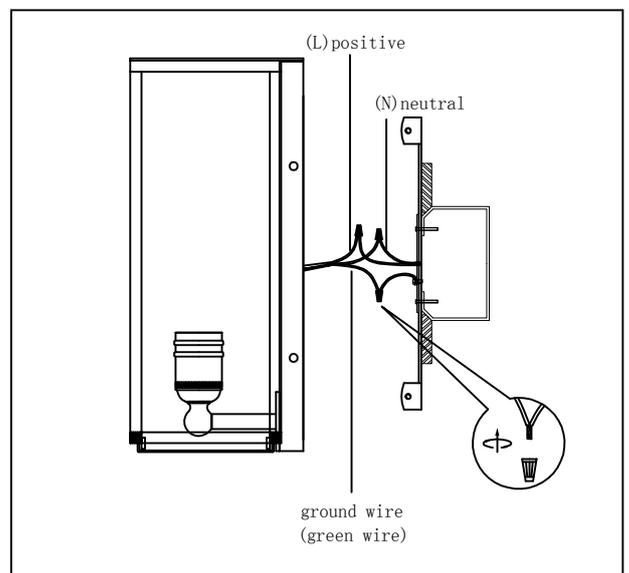
**Step.2:** Wire fixture to wires in outlet box. Copper/green wire is for Ground.
