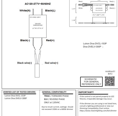
THIS FIXTURE MUST BE INSTALLED with a COMPATIBLE DIMMER SWITCH DO **NOT** CUT FACTORY-MADE CONNECTIONS.
