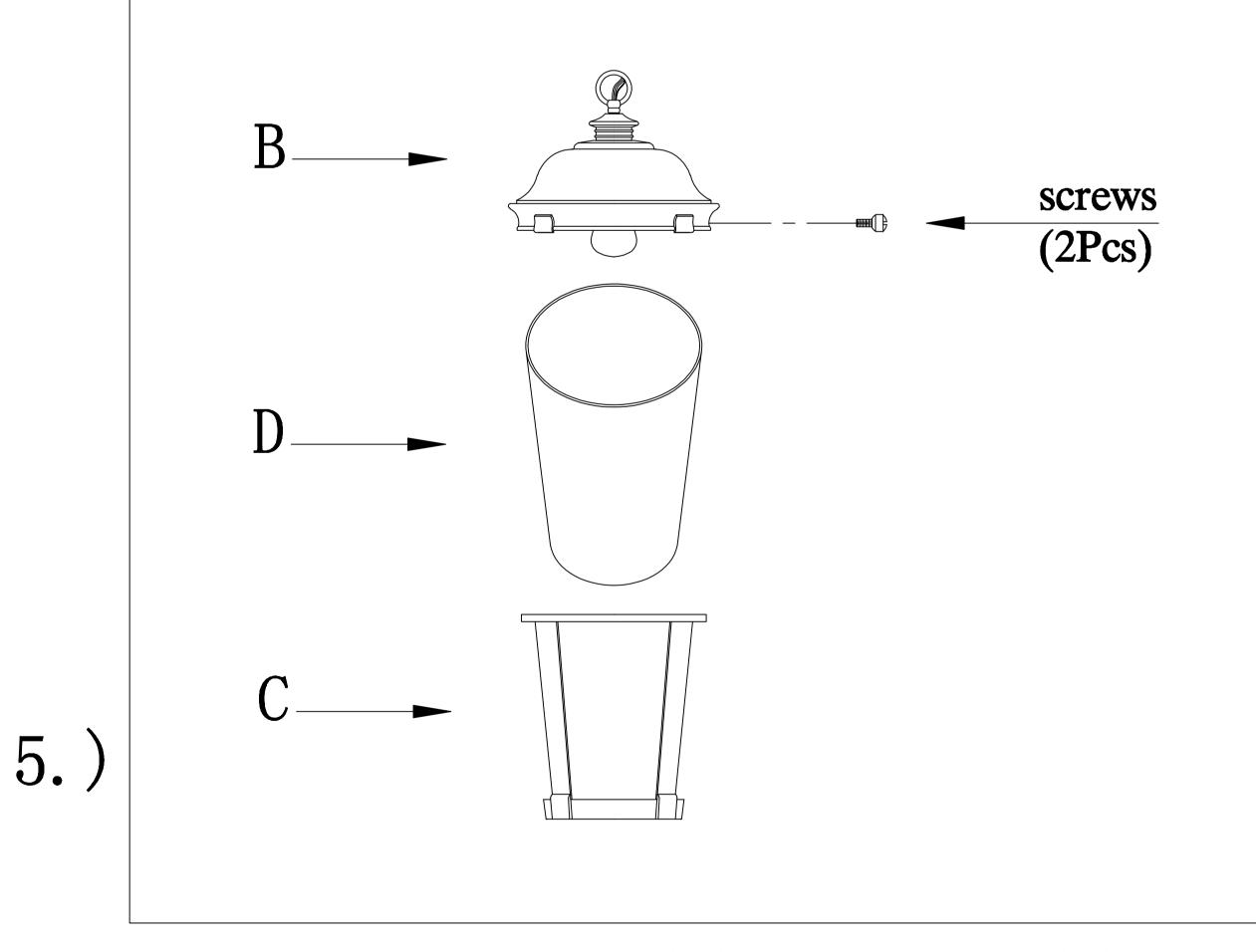
Step.5: Install the glass(D) into the cage(C), Install the cage(C) to the fixture(B) using screws.
