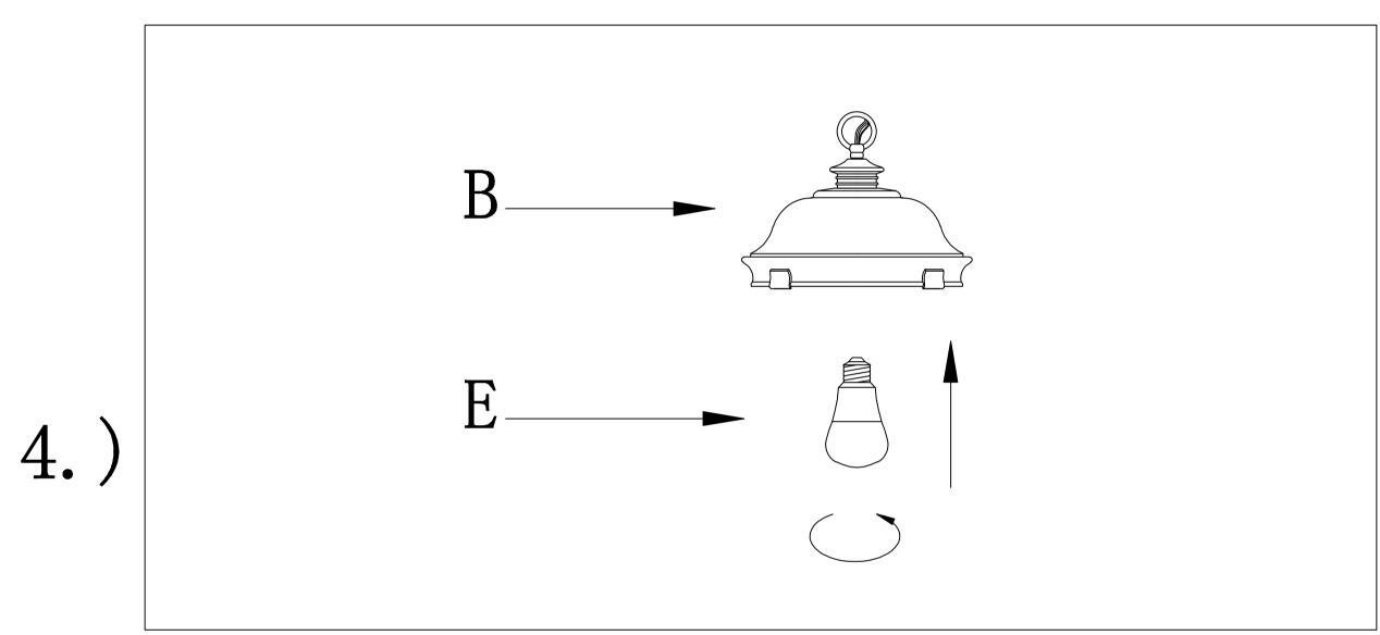
Step.4: Install E26 LED bulb(E)
