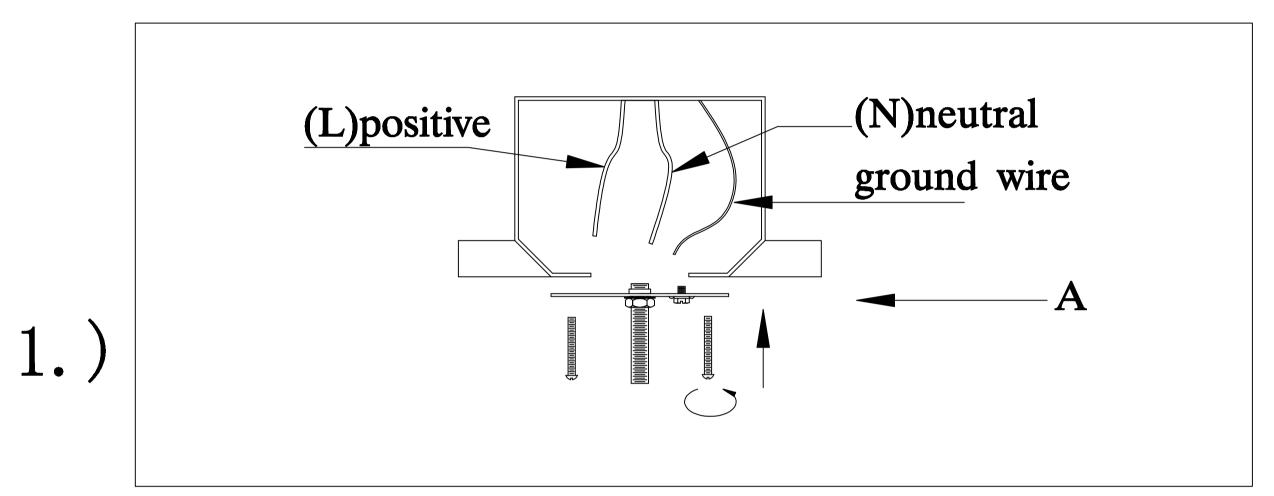
Step.1: Remove mounting bracket(A) from fixture and install to electrical box.
