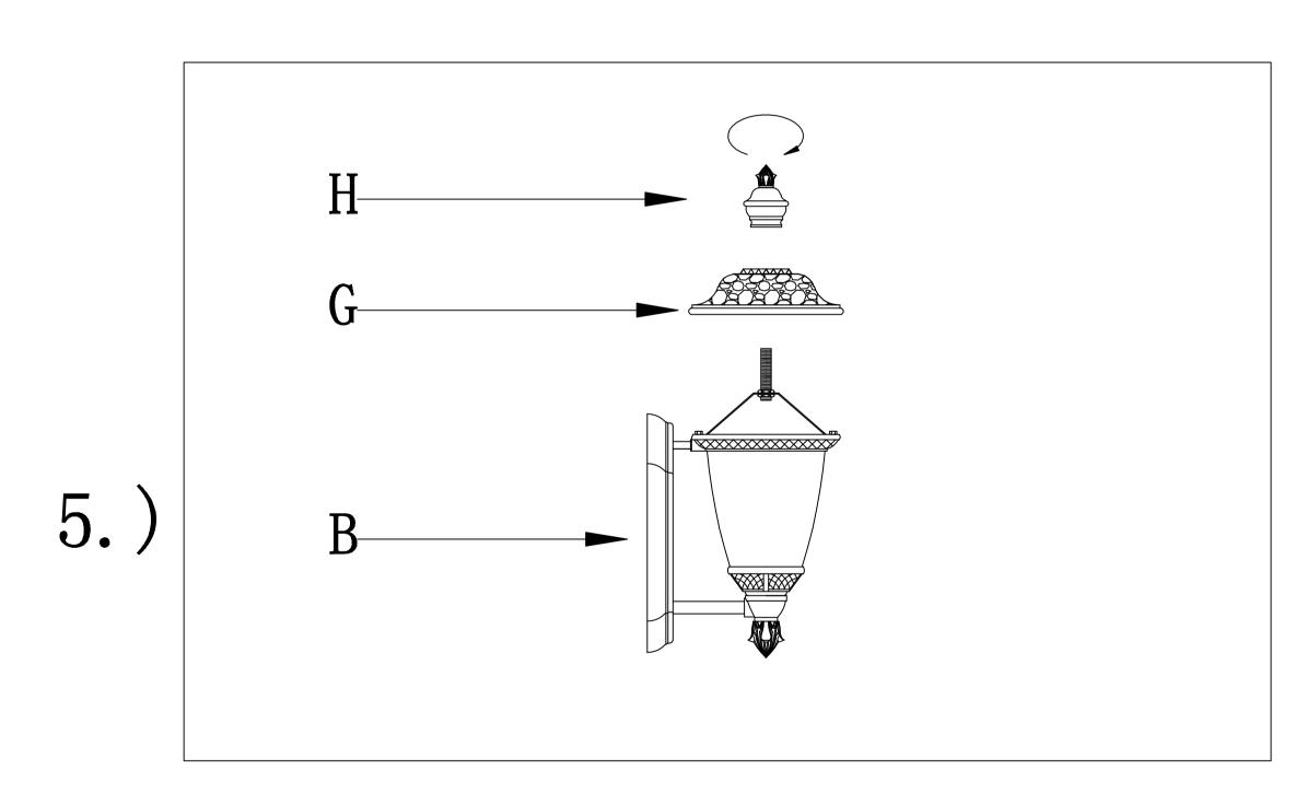
Step.5: Install the cover(G) and the finial(H) to fixture, Then tighten the finial.
