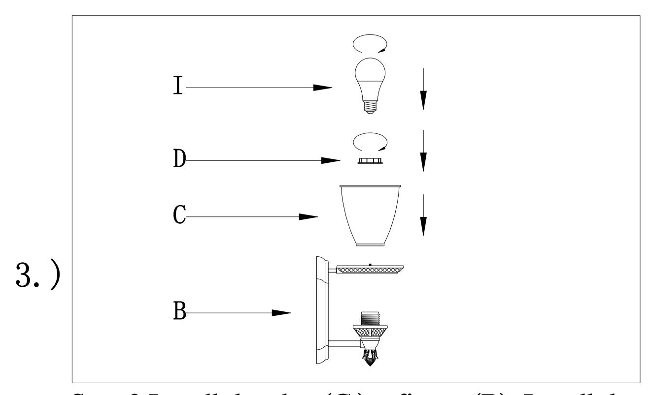
Step.3:Install the glass(C) to fixture(B); Install the screw ring(D) to fixture, tighten the screw ring; Install E26 LED bulb(I).
