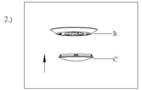
Step.2: Attach acrylic diffuser (C) to the fixture (B).
