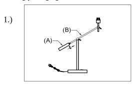
Step 1: Attach the counterweight (A) to the back end of the body (B).
