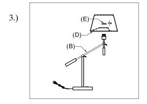
Step 3: Remove the socket ring (E) from fixture (B). Attach shade (D) and secure using socket ring (E).
