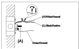
Step 2: Wire fixture to wires in outlet box. Green wire is for ground.
