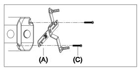
Step 1:Remove mounting bracket(A) from fixture and install to electrical box using mounting screws(C)
