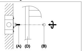
Step 3:Attach wall sconce to mounting bracket(A) and secure using decorative nuts(B) provided.
