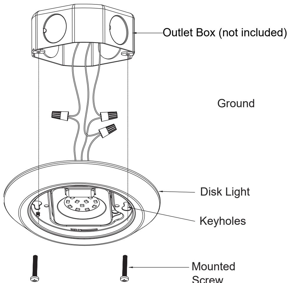
1. Install mounting screws into junction box leaving enough exposed to engage keyholes in the disk light.
