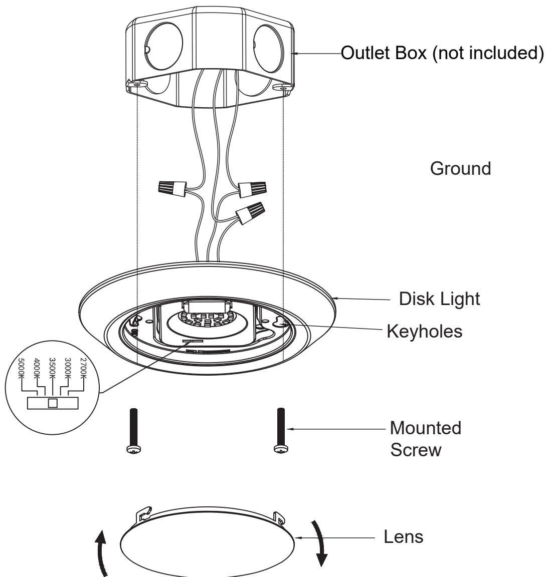
1. Install mounting screws into junction box leaving enough exposed to engage keyholes in the disk light.
