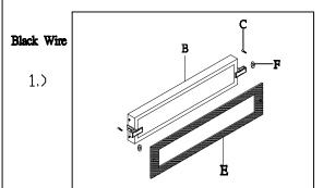
Step.1: Put the glass(E) into the fixture assembly(B), then secured by Rubber washer(F) and Ball nut(C) By the way, the Rubber washer(F) and Ball nut(C) were packed into the canopy kit
