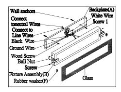
Step.2: Attach the brackets to fixture assembly (B). Slide glass (E) into brackets and secure using Screw
