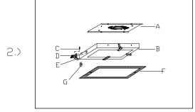
Step.1: Put the glass(F) into the fixture assembly(B), then secured by Rubber washer(G) and Ball nut(C) By the way, the Rubber washer(G) and Ball nut(C) were packed into the canopy kit
