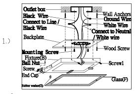
Step.2: Attach the brackets to fixture assembly (B). Slide glass (F) into brackets and secure using ball nut (C).
