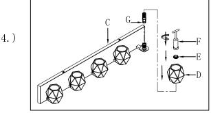
Step.4: Install G9 LED bulb(G) into socket, Position Glass(D) onto the socket of fixture body(C), then secure with socket ring(E) with Glass (D) onto Fixture body(C) by using spanner(F).
