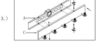
Step.3: Place the fixture body(C) against mounting bracket, Align the two holes of the mounting bracket and fixture body, then tighten the screws.
