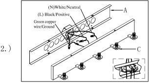
Step.2: Wire fixture to wires in outlet box. Green copper wire is for ground. And carefully position all wires inside the outlet box.
