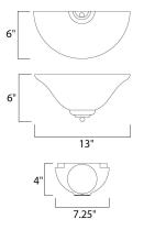
**MEASUREMENTS** DIMENSION : 13" W x 6" H x 6" Ext MAX OAH : 7.25" W x 6" H HANGING WEIGHT : 2.12 lb LAMPING INPUT VOLTAGE :120V : 1 x 60W Incandescent E26 Medium , 60W Total BULB **BULB INCLUDED** : (Not Included) DIMMABLE LIGHTING\_DIRECTION : Up
