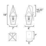
\*height from center of outlet to the top of the fixture  $% \left( t\right) =\left( t\right) \left( t$
