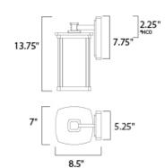
height from center of outlet to top of the fixture
