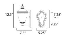
\*height from the top of the fixture to the center of the outlet
